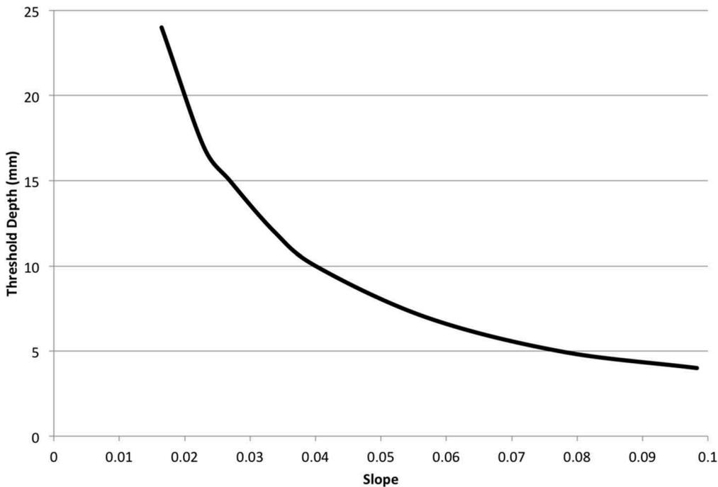
**Figure 5.** Minimum depth necessary to transport an 8 mm median diameter particle for the range of slopes shown in Table 6.
