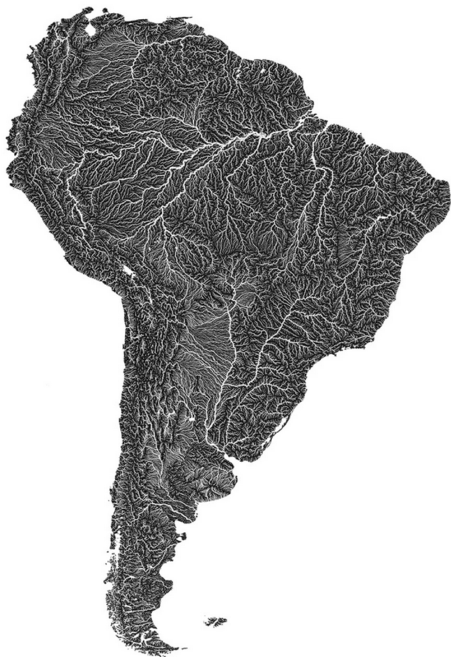
Fig. 1. Continental scale surface drainage of South America. The map shows stream segments, with width proportional to Strahler order. Map produced by Jared Prince, Muir-Way ( https://muir-way.com ) and used by permission.
