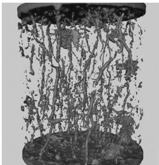
Fig. 2. Macropores ( \geq 0.6 mm) revealed by CT scanning of soil core 20 cm in diameter by 20 cm tall from a loamy soil in Denmark. Imaging by Dorthe Wildenschild, modified from a figure shown at https://www.producer.com/crops/ct-scan-tech-used-to-check-soil-health/ .
