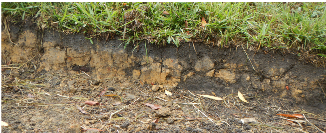
Fig. 8. Soil in southeast Queensland, Australia originally formed under subtropical forest. Segregated dark areas and visible partings show macropores, looser subsurface material, and buried organic matter pockets that become connected during wet periods.
